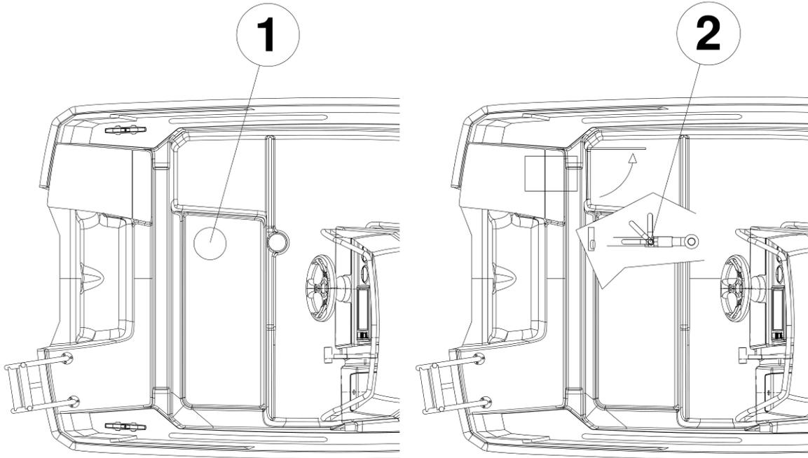
1. The maintenance hatch for the rainwater drainage valve and for the drainage pump (the pump is an optional accessory)
