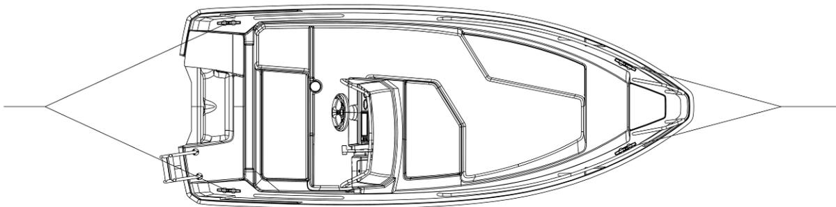
Attaching the towline to the bollards.
