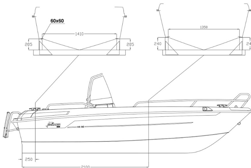
Only use reputable lifting companies or boat yards with sufficient lifting capacity. In addition to the boat's tare weight (please refer to the technical specification), also take into consideration accessories and other possible loads in the boat.
