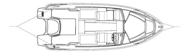
Image: Location of anchoring bollards during towing.
