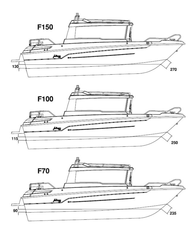
Image: Boat's antifouling measurement points.
